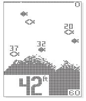
allows you to determine the texture and relative hardness of the bottom. Selecting Bottom Black "ON" causes the unit to blacken in the display below the bottom. This gives the user easiest recognition of the bottom location, even from a great distance.
